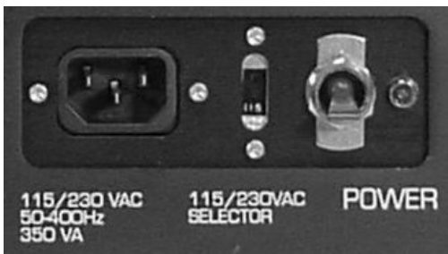
Power Switch/Circuit Breaker Lower Right Corner - Controller Back Panel
