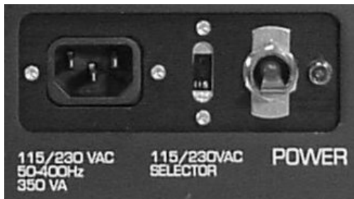
Power Switch/Circuit Breaker Lower Right Corner - Controller Back Panel
